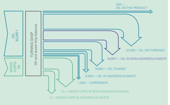
FIGURE 14: Complete balance of turning oil and wood chips in manufacturer of ball bearings
