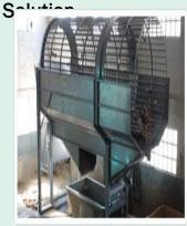
The process involves pounding the skins to reduce the amount of salt needed for salting. Experience has shown that using this option for pollution prevention can reduce the amount of about 6 to 8% of the salt content, amounting for 5% of the salts released by the tannery.
