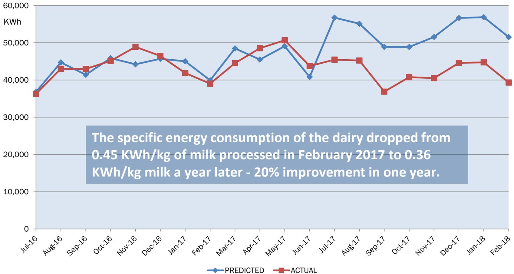
The specific energy consumption of the dairy dropped from 0.45 KWh/kg of milk processed in February 2017 to 0.36 KWh/kg milk a year later - 20% improvement in one year.
