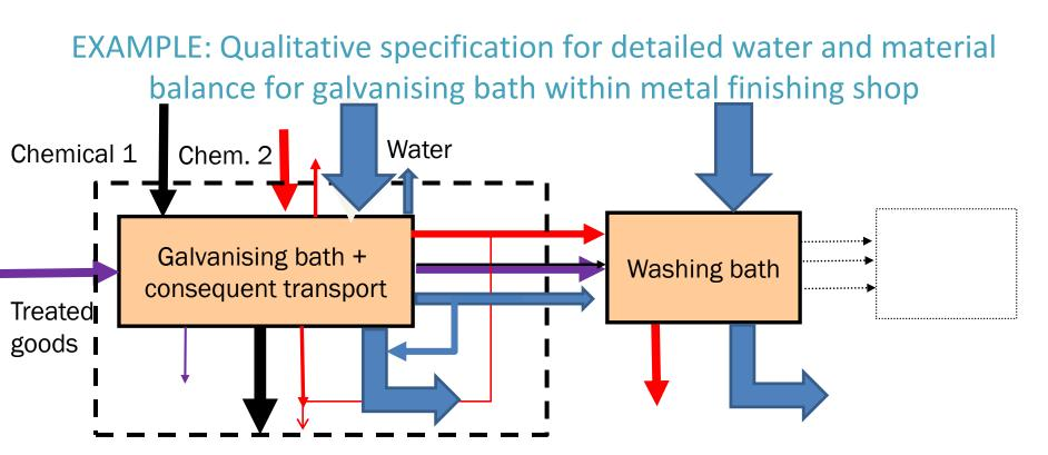
**Detailed balance for galvanising bath and transport to the next bath:** (balance borders are highlighted by dashed line; all flows should be quantified within the next step)
